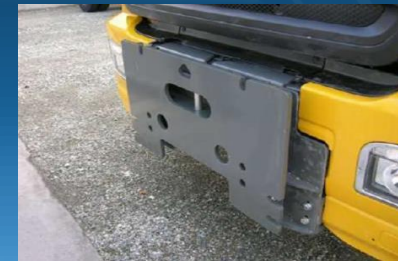
Enhanced with plate spring to reserve a snow shovel mounting port
