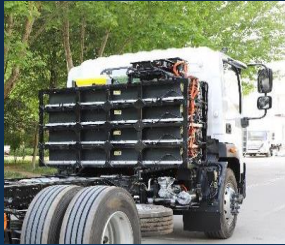
Lithium iron phosphate 246/282 kWh large capacity battery
