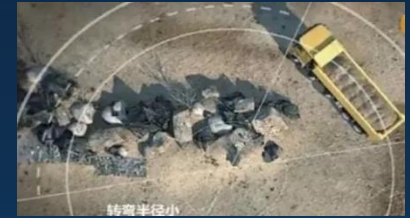
The turn signal of the front axle increases to 41^{\circ} , realizing a small turning radius
