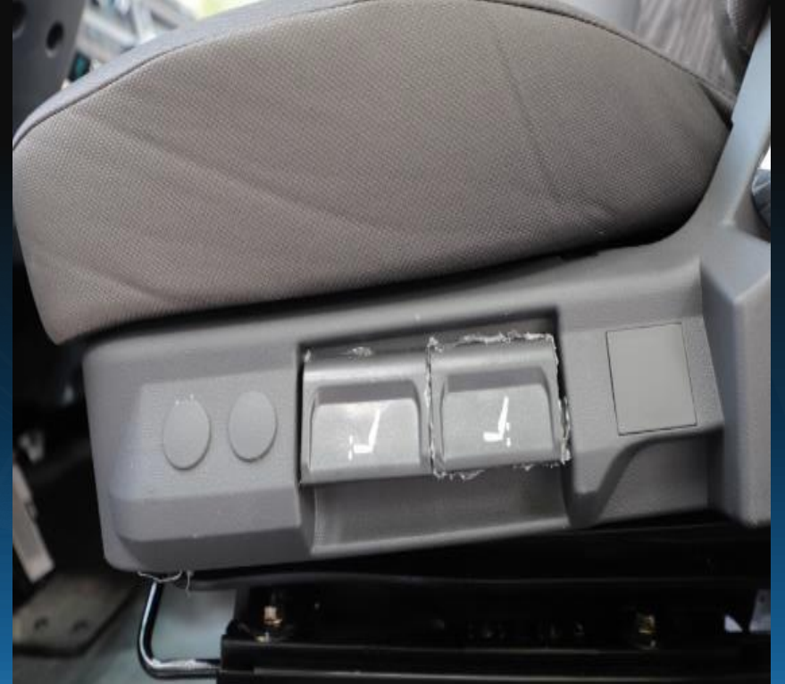
Adjustable airbag seat (forward and backward), and adjustable backrest angle
