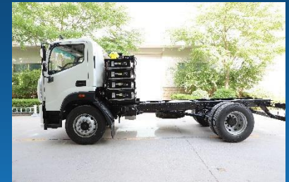
Center shifting forward, ensuring rational front and rear axle load distribution
