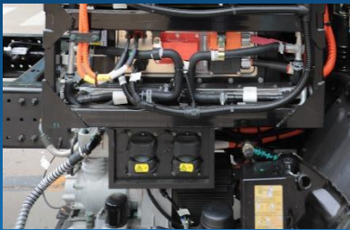
Dual charger fast charging, with the maximum charging current reaching 400A, reducing charging time
