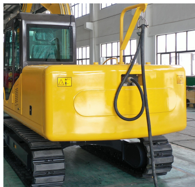
Cable Power Supply
