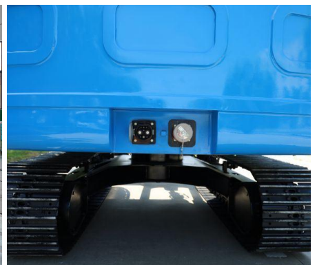
Lithium Battery Power Supply
